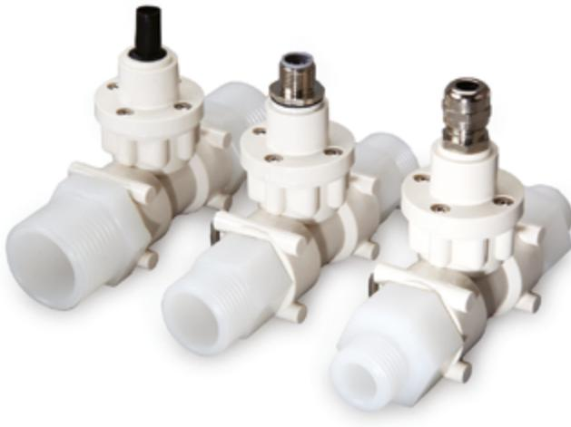
This multi-range radial flow turbine meter uses a low inertia turbine supported on robust sapphire bearings in a chemically resistant housing. Nine flow ranges (0.02 to 160 L/min), a choice of 'plug in' fittings and individual traceable calibration, make this meter one of the most flexible available.
