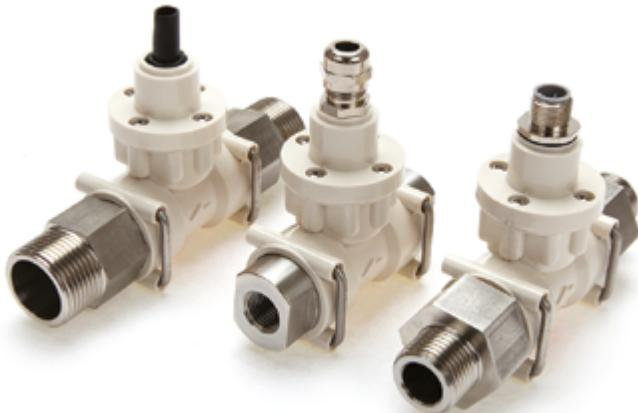
This multi-range radial flow turbine meter uses a low inertia turbine supported on robust sapphire bearings in a chemically resistant housing. Nine flow ranges (0.05 to 160 L/min), a choice of 'plug in' fittings and individual traceable calibration, make this meter one of the most flexible available.
