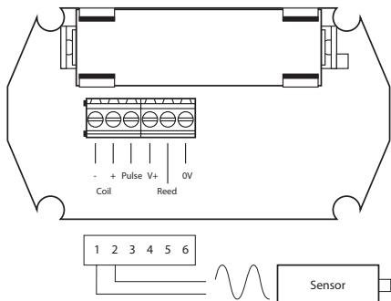
**External power.** Installations with contact closure or magnetic pick-ups can also operate with external power. For powered sensors external power should always be used.
