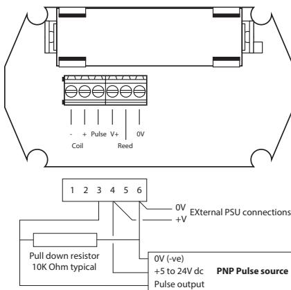
**Logic level & TTL interface.** 2KHz Max. External power not essential but recommended.
