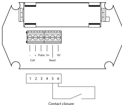
**Magnetic pick-up.** 3mV to 24V peak to peak sine wave. 2KHz max.
