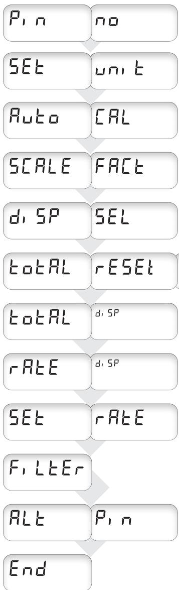
Holding both buttons for a minimum four seconds enters the menu system.
