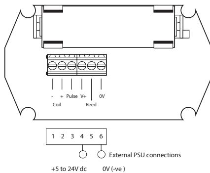
**NPN pulse i.e. Hall effect sensor.** 2KHz. Max. This input would require external power.
