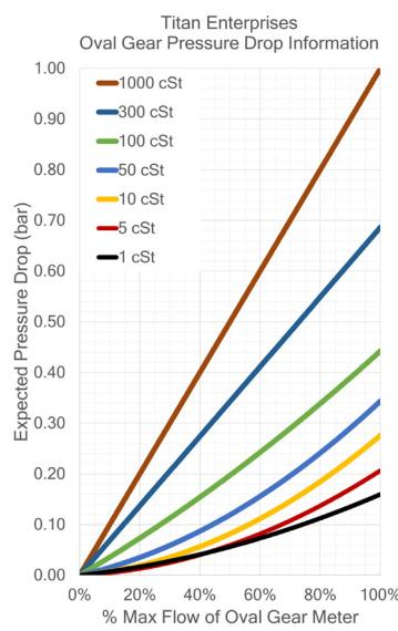
The rugged OG6 oval gear flowmeter is designed to give high performance with a low cost of ownership. It has a standard flow range from 2.0 to 200 L/min on 30 cSt oil and 10 to 200 L/min on water-like liquids. The standard inlet and outlet are 1½" female threads. For OEMs, alternatives are available, including manifold mountings. The standard models are 316 St St or Aluminium with Viton™ 'O' ring seals.
